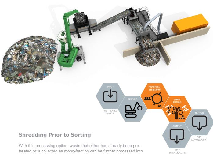
treated or is collected as mono-fraction can be further processed into a substitute fuel with high quality. After shredding, the material can be further separated with a windsifter. Low density, flat objects are extracted while heavier, more compact particles remain on the belt.
