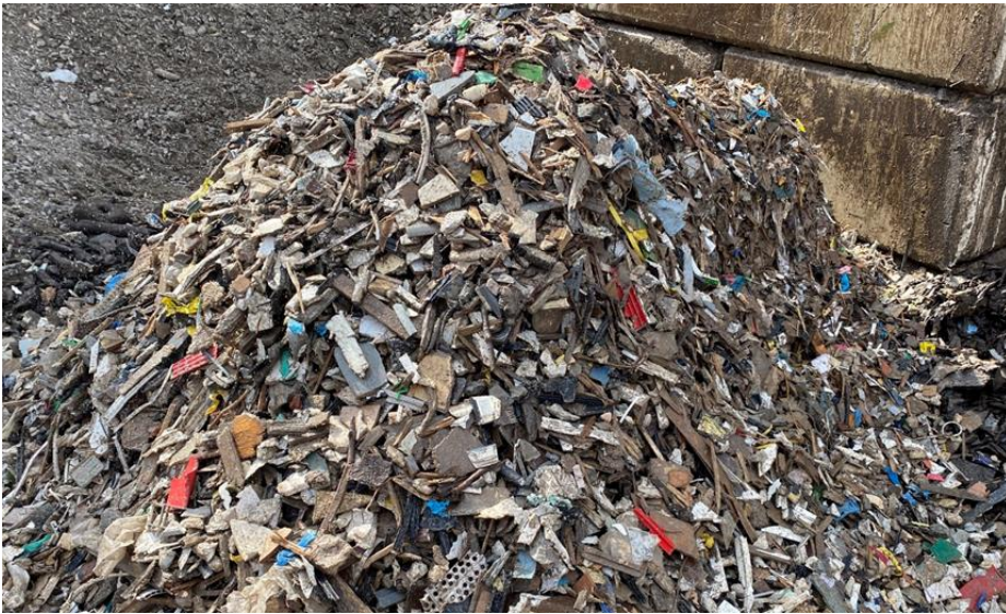
Mixed pre-shredded waste largely < 300 mm
