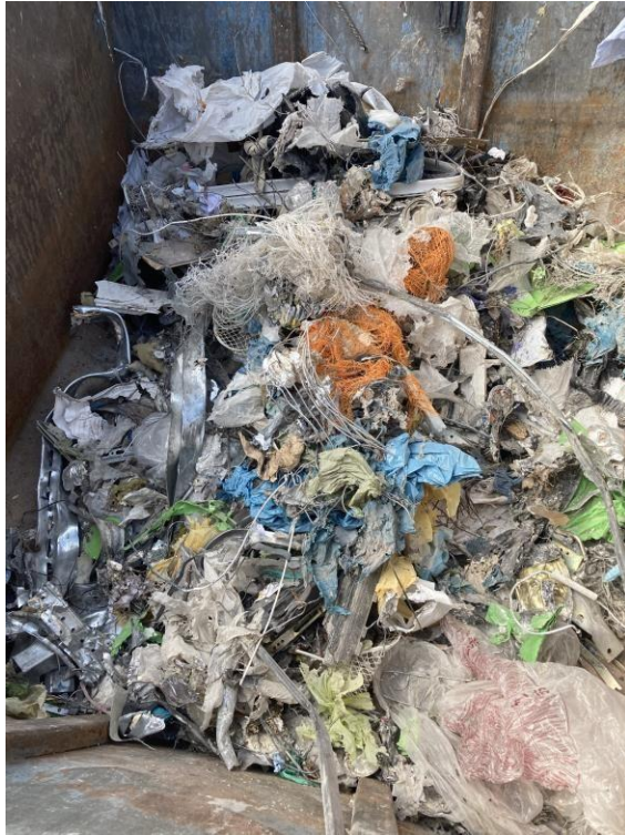
Fe fraction – extracted with the magnet
