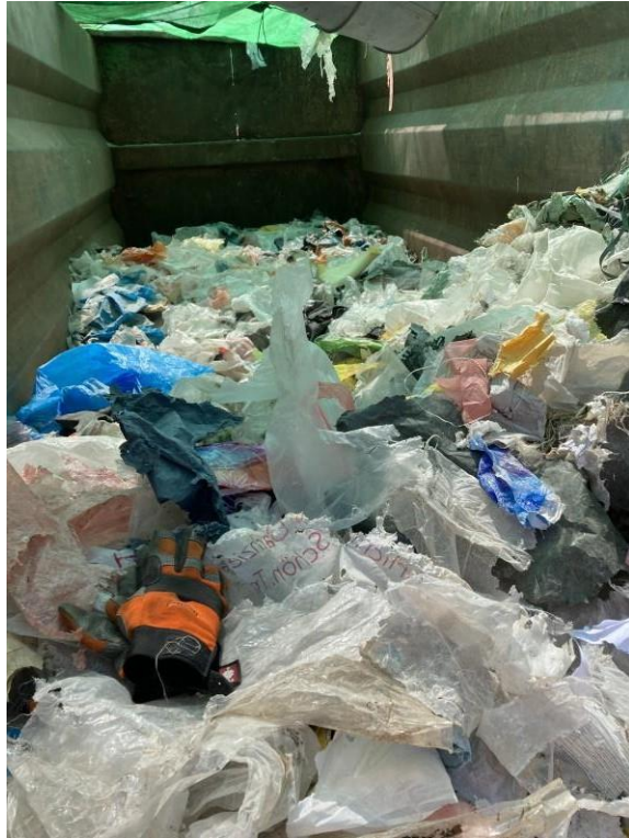
Foil fraction obtained with the windsifter
